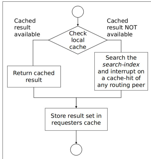
Fig. 5. Search process & cache generation flow chart
