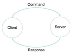
Fig. 3 Message exchange between a Client and a Server
