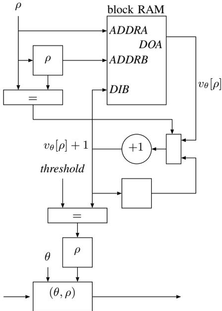
Figure 7. A block RAM  $V_\theta$  to store  $v[\theta][\rho]$
