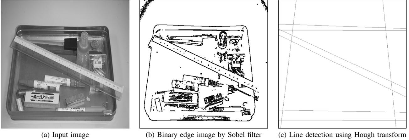
Figure 1. Example of straight line detection using Hough transform
