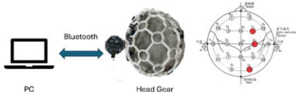
Fig. 6. Overview of EEG Measurement System and Electrode Arrangement Diagram
