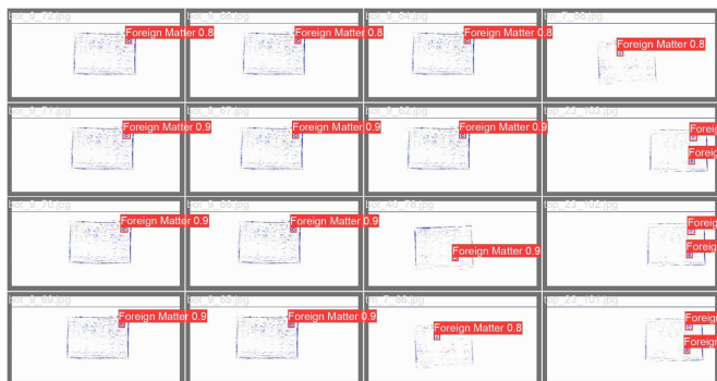
Figure 3. Result of foreign matter detection within seaweed using the trained model's weight file.
