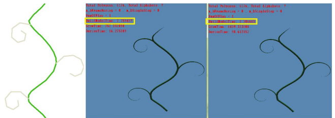
Figure 6. On the left is the current system interface for input; in the middle simulates the plant growth by Simeco without CUDA; to its right simulates plant growth by Simeco with CUDA.
