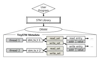
Fig. 3. TinySTM structure on DRAM
