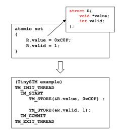
Fig. 2. TinySTM example source code
