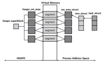
Fig. 1. Process Address Space in HEAPO
