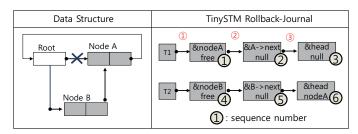
Fig. 5. Sequence number to manage recovery: (1)Alloc Node and Copy K-V,(2)Write Pointer,(3)Update Pointer
